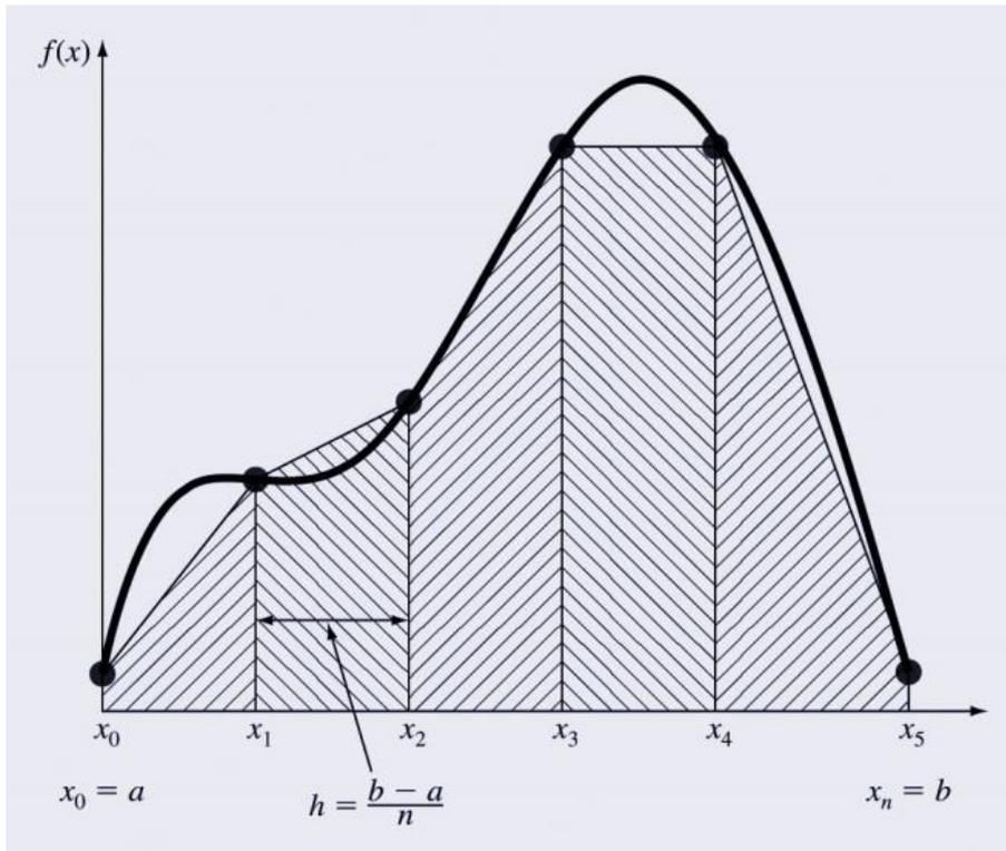
$$I \cong \underbrace{(b-a)}_{\text{ancho}} \underbrace{\frac{f(x_0) + 2 \sum_{i=1}^{n-1} f(x_i) + f(x_n)}{2n}}_{\text{altura promedio}}$$
