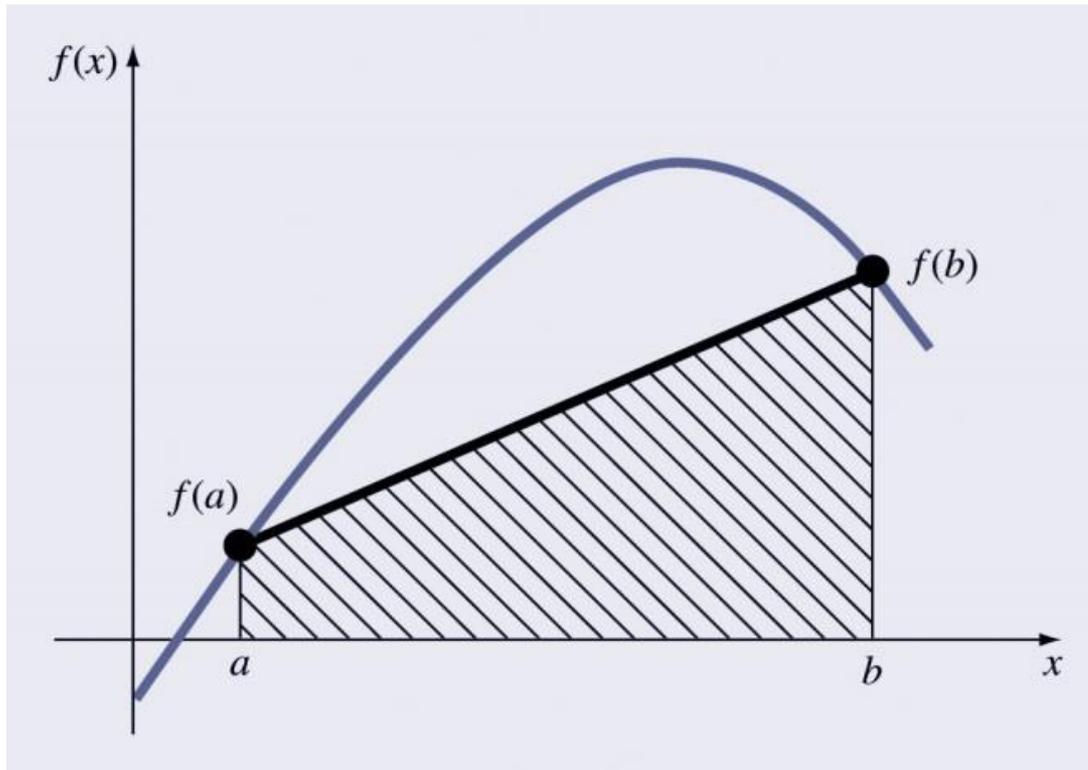
$$I \cong \underbrace{(b-a)}_{\text{ancho}} \underbrace{\frac{f(a)+f(b)}{2}}_{\text{altura promedio}}$$
