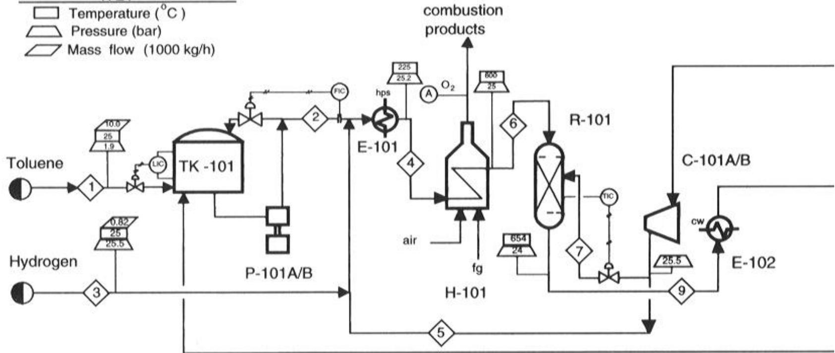
Benzene process flow diagram (PFD) for the production of benzene via the hydrodealkylation of toluene.
