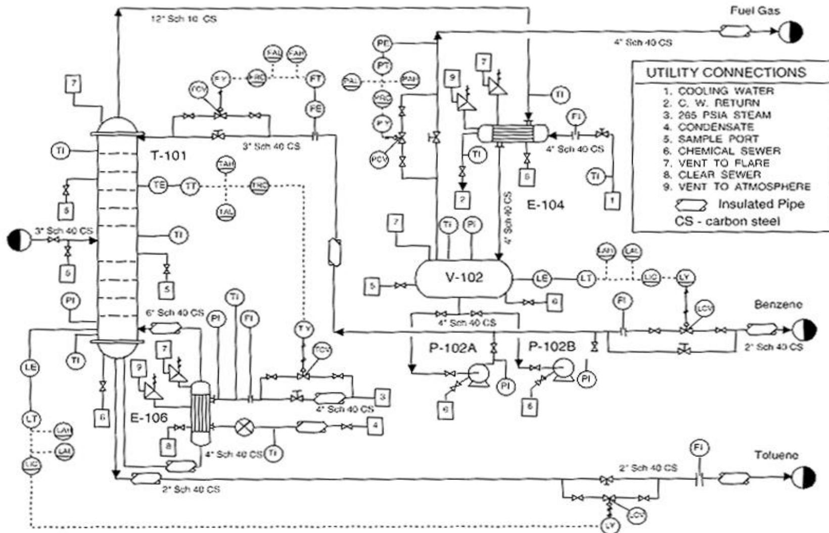
**Figure 1.7** Preliminary piping and instrumentation diagram for benzene distillation. (Adapted from Kauffman, D., *Process Sheets and Diagrams*, AIChE Modular Instruction, Series G: Design of Equipment, series editor J. Beckman, AIChE, New York, 1986, vol 1, Chapter G.1.5, AIChE copyright, © 1986 AIChE, all rights reserved)
