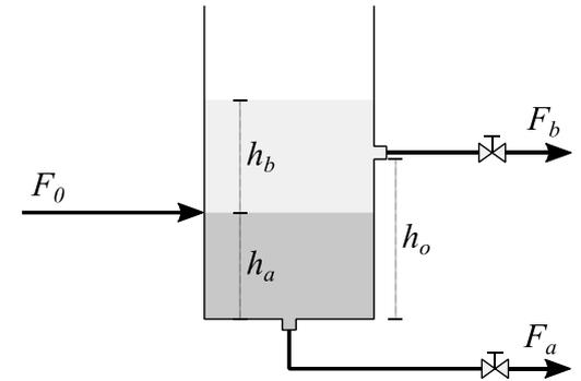
$$F_b = C v_b \sqrt{\frac{\Delta P_b}{\rho_b}} \quad \rightarrow \quad \Delta P_b = P_0 + \rho_b g (h_a + h_b - h_o) - P_0$$
