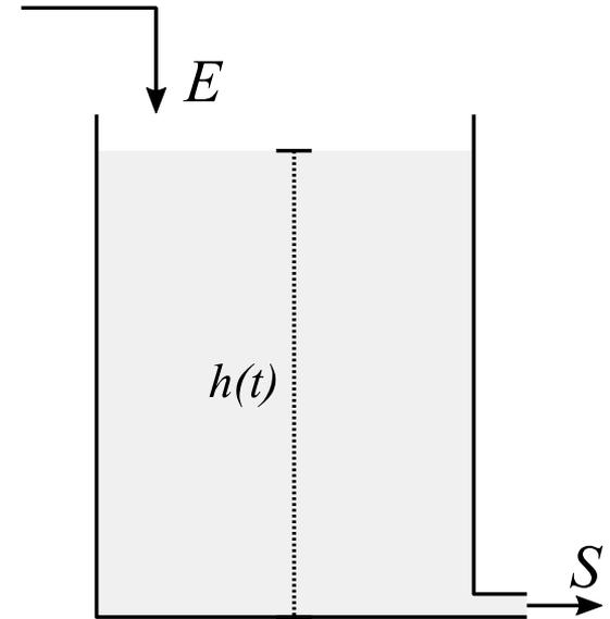
$$A_T = \frac{\pi D_T^2}{4} \quad A_s = \frac{\pi D_s^2}{4} \quad \rightarrow \quad A_T \frac{dh}{dt} = -A_s \sqrt{2gh} \quad \rightarrow \quad \frac{\pi D_T^2}{4} \frac{dh}{dt} = -\frac{\pi D_s^2}{4} \sqrt{2gh}$$
